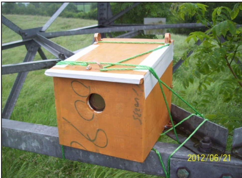
Figure 3.6a: The purpose built 'mock' bird nesting box with the AnaBat SD2 microphone positioned at the front opening.
