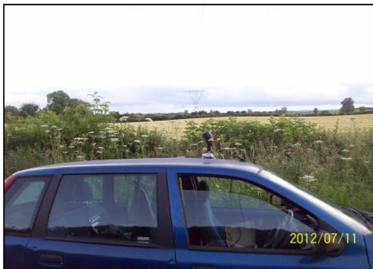
Figure 3.2: Survey vehicle with Anabat microphone mounted on car roof
